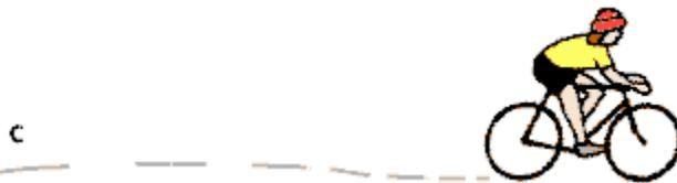
c) Achieve a quick stop by squeezing the front brake three times as hard as the rear brake. If the rear wheel skids, reduce force on the front brake.
