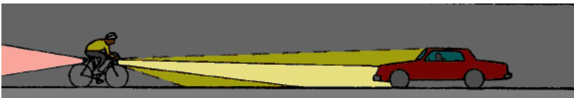
Mount a generator or high-powered battery light low, so its beam pattern extends longest and reveals surface irregularities.
